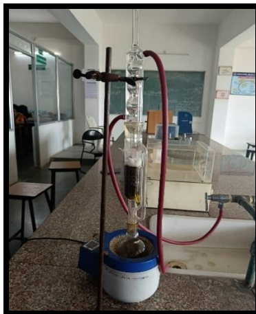
Figure 2: Extraction of Piper nigrum by Soxhlet apparatus
