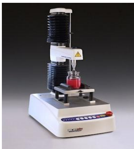
Figure 2: Mechanism of determination of gel strength
