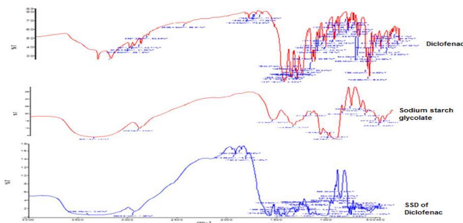
Fig. 3. Comparative FTIR spectra of Diclofenac, Sodium starch glycolate & Surface solid dispersion of Diclofenac
