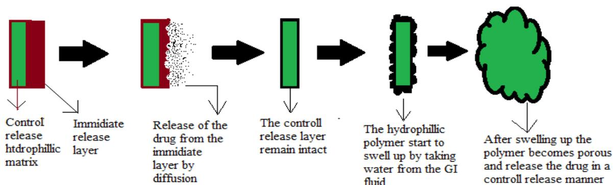
Figure 3: DUREDAS technology consists of control release and immediate release layer.
