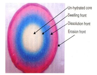
**Figure** 1: Hydrophilic matrix containing drug after hydration for 8 hours in cobalt (II) thiocynate solution. The white region is the unhydrated core, blue region is the hydrated region-containing drug and pink region is the drug free hydrated polymer
