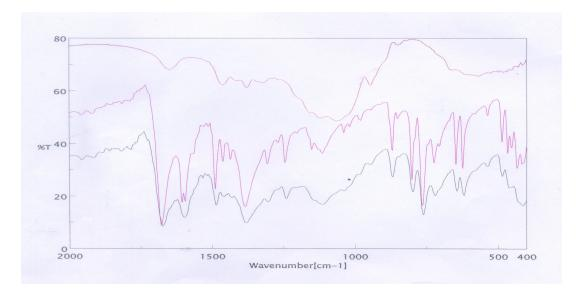
Figure 5: IR Spectrum of Carbamazepine, HPMC, Carbamazepine + HPMC
