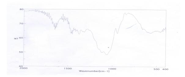
Figure 4: IR Spectrum of HPMC (Hydroxy Propyl methyl Cellulose)
